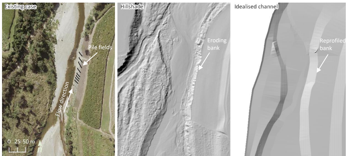
Figure 35. O'Connell River Site 2 showing the existing pile field design (left), hillshade of the pre-works terrain (middle), and the of36alized terrain model.
