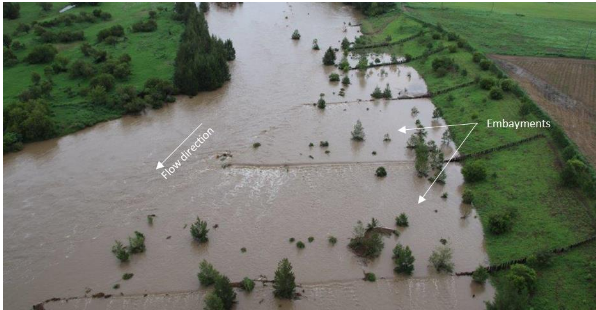
Figure 5. Permeable pile fields along Upper Brisbane River, Harlin, showing reduced flow velocities within embayments.
