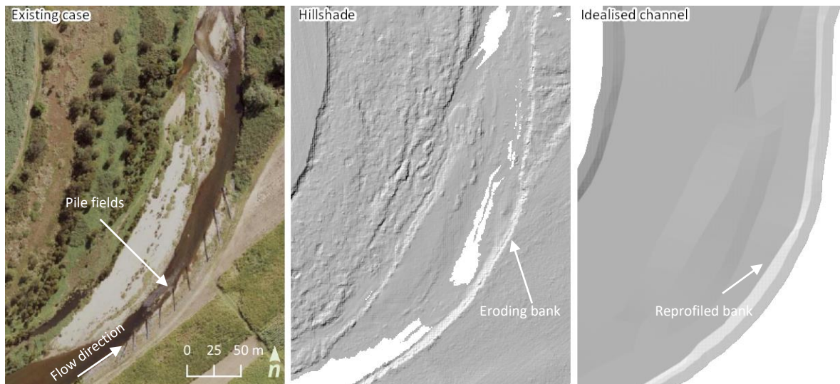
Figure 36. St Helens Creek site showing the existing pile field design (left), hillshade of the pre-works terrain (middle), and the of36alized terrain model.
