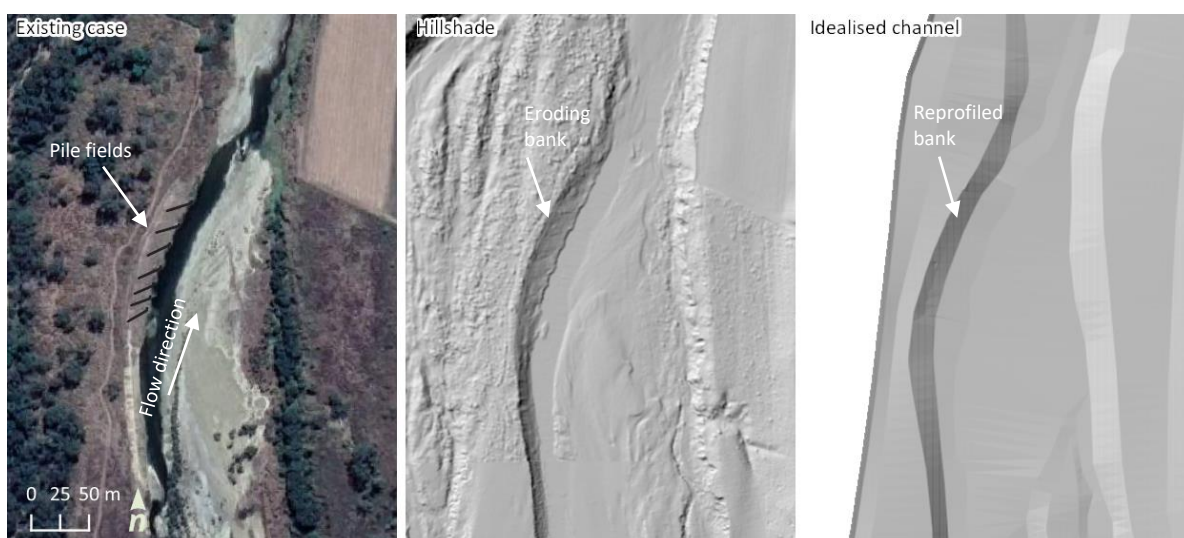
Figure 34. O'Connell River Site 1 showing the existing pile field design (left), hillshade of the pre-works terrain (middle), and the of35alized terrain model.
