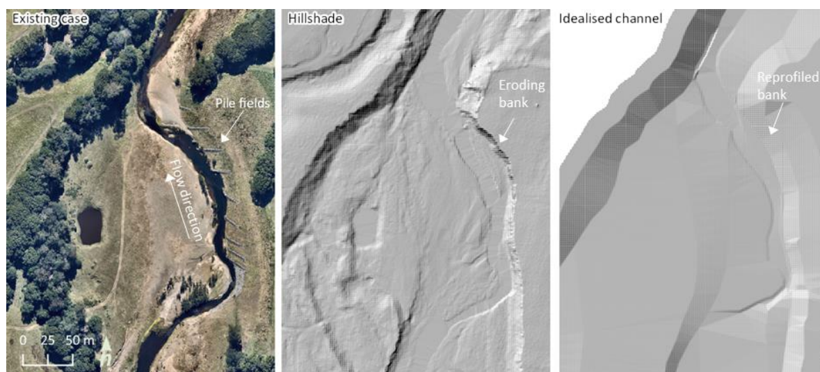
Figure 33. Mary River Carters site showing the existing pile field design (left), hillshade of the pre-works terrain (middle), and the of35alized terrain model.
