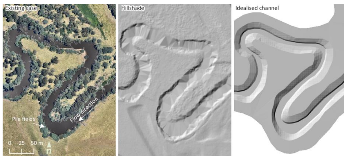
Figure 38. Yarra River site showing the existing pile field design (left), hillshade of the pre-works terrain (middle), and the of37alized terrain model.
