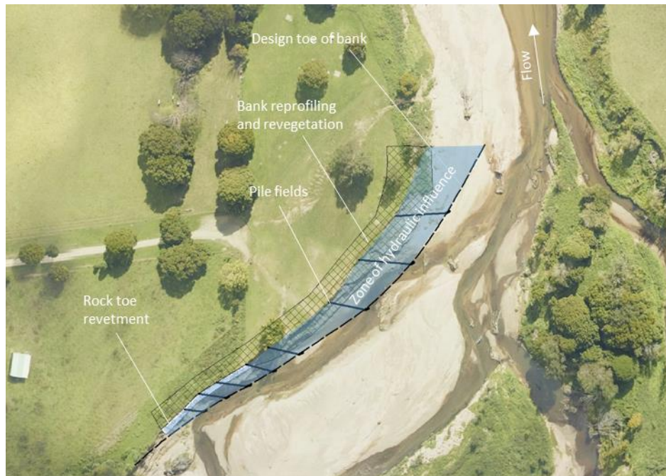
Figure 61. Example pile field design showing the design toe of bank set out from toe of the bank and the zone of hydraulic influence.
