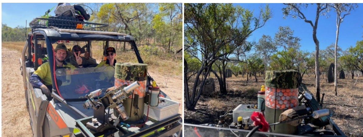
Figure 31 Prescribed fire lighting unit that can shoot incendiary balls 50 m from tracks to create effective firebreaks and rotate the location of annual burning (courtesy of Tropical Fire Technologies, Darryl Killin).
