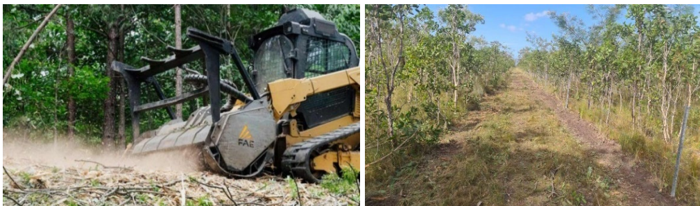
Figure 25 Use skid steer mulchers for clearing saplings and small trees from fences and firebreaks.
