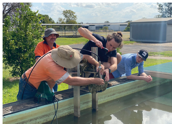
DIN sensor prototype installation for a limited tank trial at the Hydrographic Support Unit at Rocklea, IntelliDesign.
