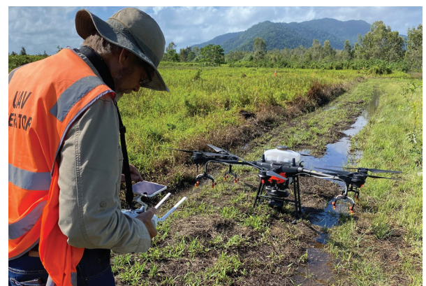
Drones were used for vegetation and germination assessments, monitoring, weed treatment, and seeding at the riparian and low-lying wetland trial site, Greening Australia.
